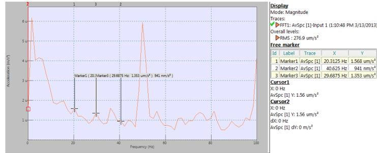
Figure 2: Vibration Spectrum of 0.2 mm – Nitrile Butadiene Rubber- 600 r.p.m. - Horizontal Direction
