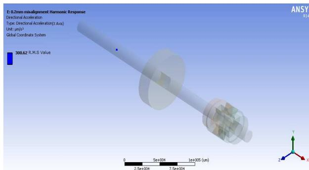
**Figure 5: R.M.S Value of Acceleration for 0.2 mm Parallel Misalignment with Elastomer as Hytrel and Speed 600 r.p.m**
