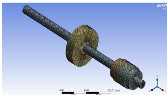
**Figure 4: Meshed Model of Shaft, Disc and Coupling Assembly**
