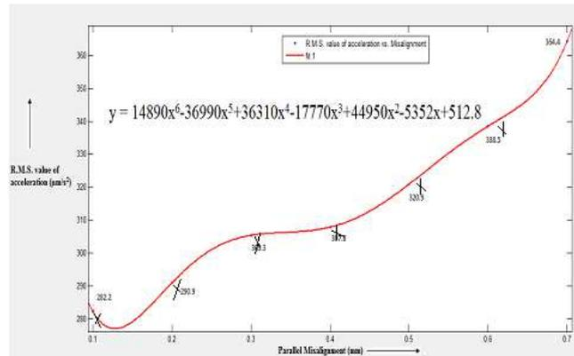
**Figure 3: Curve Fitting for 600 R.P.M., Parallel Misalignment, Polyurethane Elastomer in Horizontal Direction**
